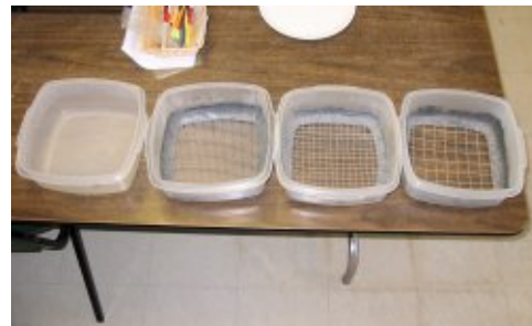
Figure 9.16. Disassembled set of screens. Left to right: Bottom tray (no mesh), 1/4-inch mesh, 1/2-inch mesh, and 1-inch mesh.
