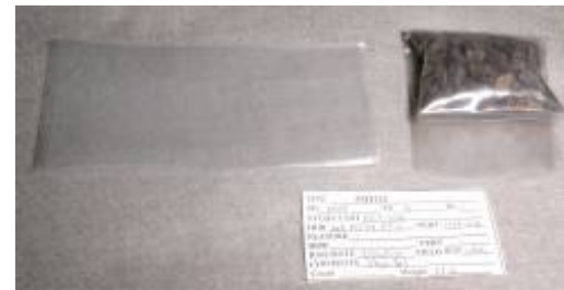
Figure 3.65. A vegetal sample ready for double bagging. The folded bag with charcoal will be inserted into the bag on the left, and the label will be placed between the two bags.
