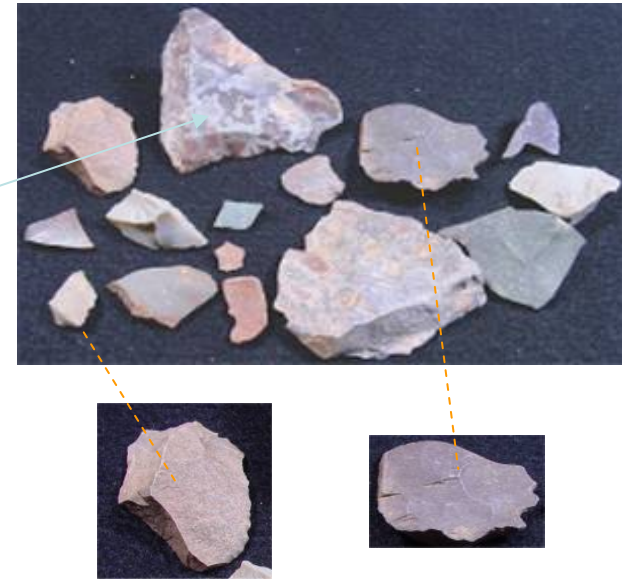
Figure 8.3. Morrison silicified sandstone. Note the mottled colors; close-up views show a rougher sample on the left and a somewhat smoother sample on the right.
