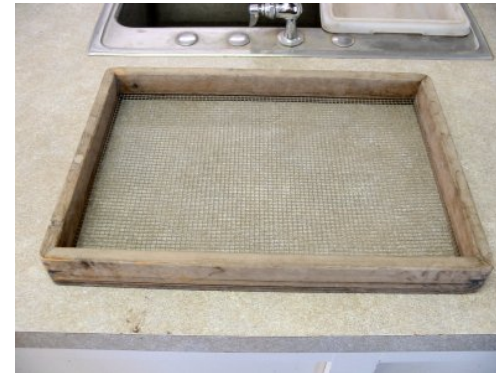
Figure 11.2. Drying screen (with \frac{1}{4} -inch hardware mesh).
