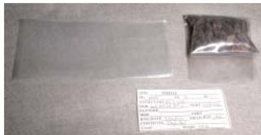
Figure 3.63. A vegetal sample ready for double bagging. The folded bag with charcoal will be inserted into the bag on the left and the label will be placed between the two bags.
