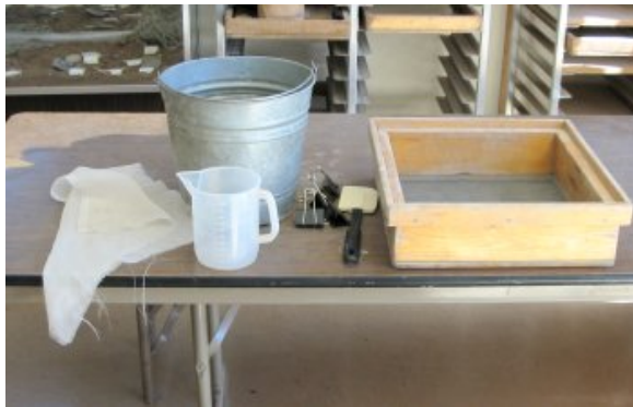
Figure 11.1. Flotation equipment. Left to right: 0.355-mm mesh wedding veil, a bucket, a graduated cylinder, binder clips, a spatula, and a sink-fitting screen with \frac{1}{4} -inch hardware mesh.
