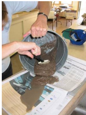
Figure 11.18. Scooping the heavy fraction onto a newspaper-lined tray to dry.
