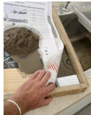
Figure 11.19. Placing the FS label under the heavy fraction.
