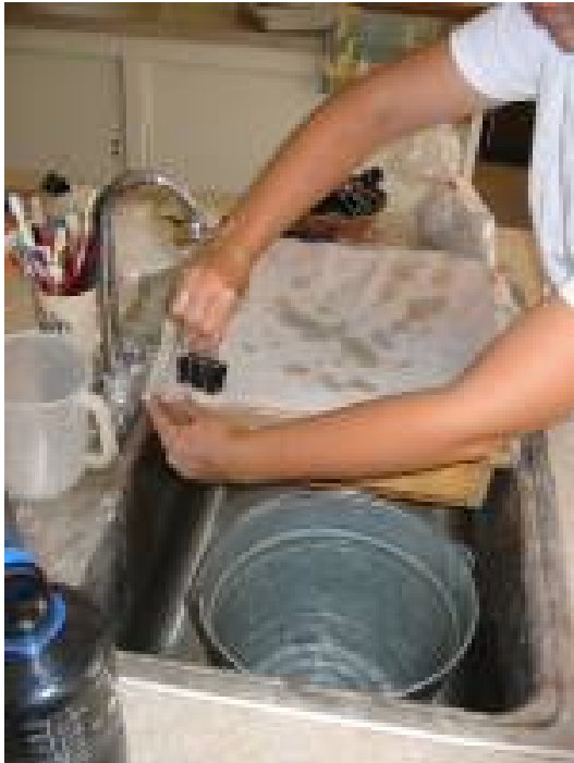
Figure 11.10. Using binder clips to attach the mesh to the sink-fitting screen.
